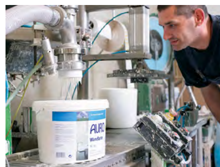
Wall paint filling
