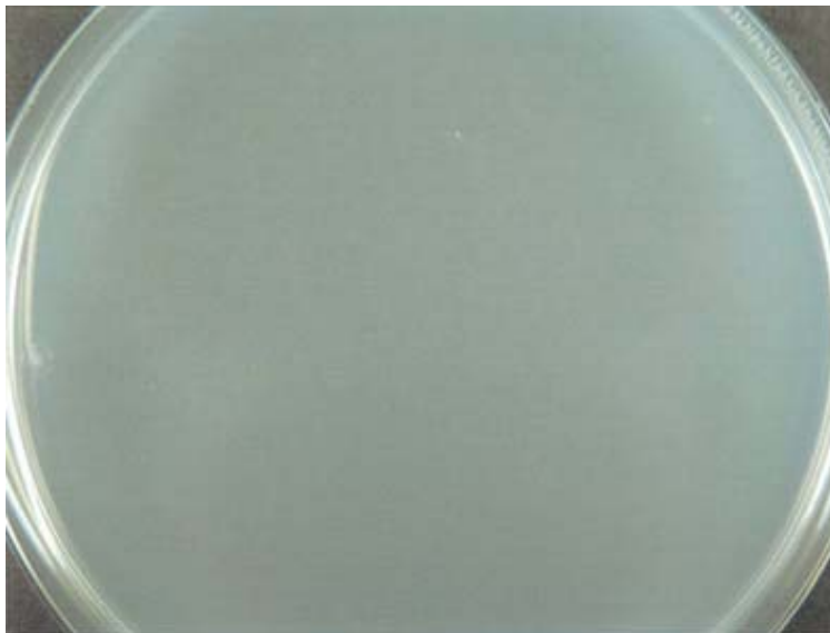
Photo 6 Penicillium citrinum , cultivation on AURO No.413 Anti-mould treated test sample, 4 th week.
