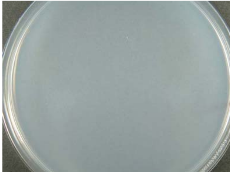
Foto 2 Aspergillus niger , cultivation on AURO No.413 Anti-mould treated test sample, 4 th week.
