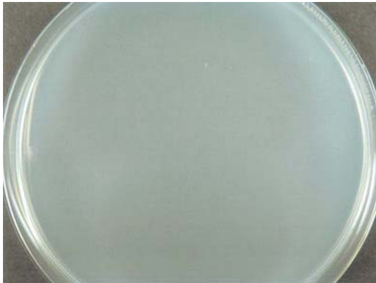
Photo 4 Cladosporium cladosporioides , cultivation on AURO No.413 Anti-mould treated test sample, 4 th week.
